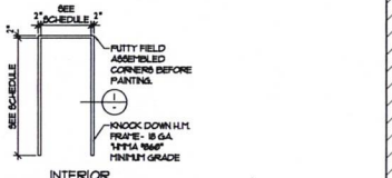
F1 INTERIOR HALF FRAME DOOR NOT TO SCALE D2 INT. WOOD DOOR NOT TO SCALE
